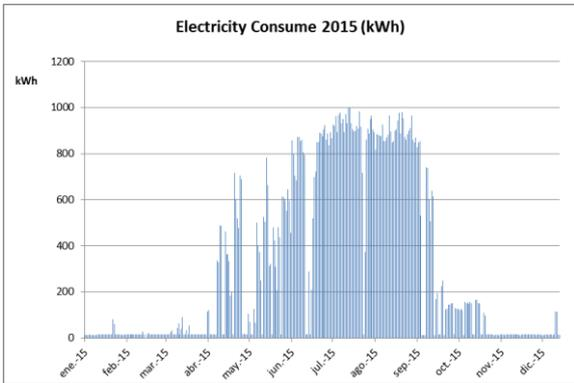
Fig. 5. Electricity consume associated to pumping corresponding to 2015
