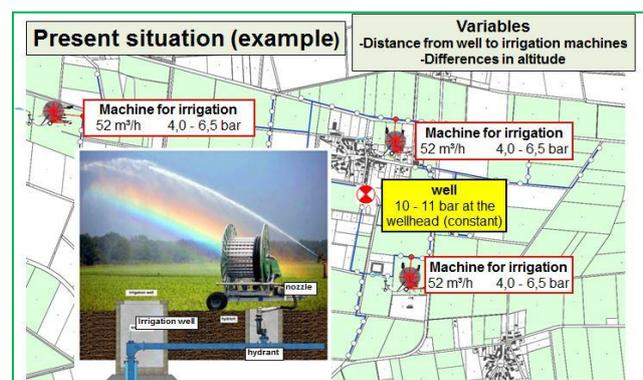
During this case, a comparison of the required pump capacity for two different pressures at the wellhead took place in order to show potential of energy saving through well regulation.
