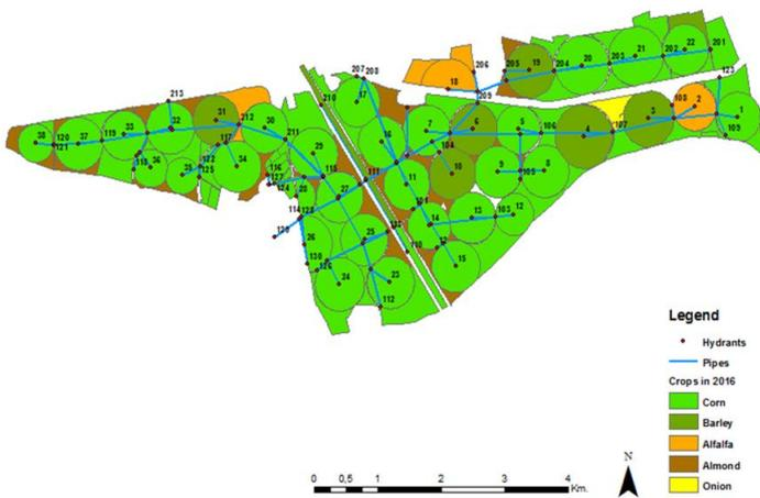
Two pumping stations at different levels supply the water to the hydrants. One pumping station with 8 pumps with capacity of 1.538 l/s (irrigates 88% of the total area) and the second pumping station with 5 pumps with of 229 l/s (irrigates 12% of the total area).
