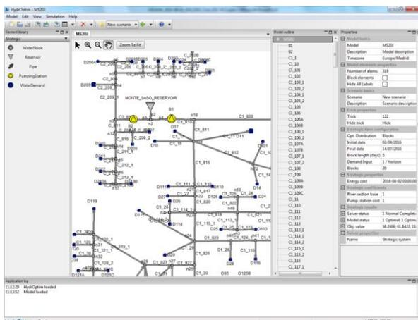
The hydraulic topology of Monte Saso sector was introduced in HydrOptim, and the different elements were configured.
